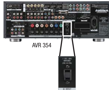
Figure 35 – Switched AC Accessory Outlet
